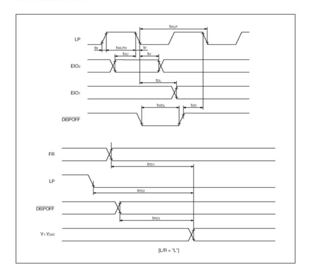
$(VSS = V5 = 0 \text{ V}, VDD = +2.5 \text{ to } +5.5 \text{ V}, V0 = +15.0 \text{ to } +42.0 \text{ V}, TOPR = -20 \text{ to } +85 ^{\circ}C)$
